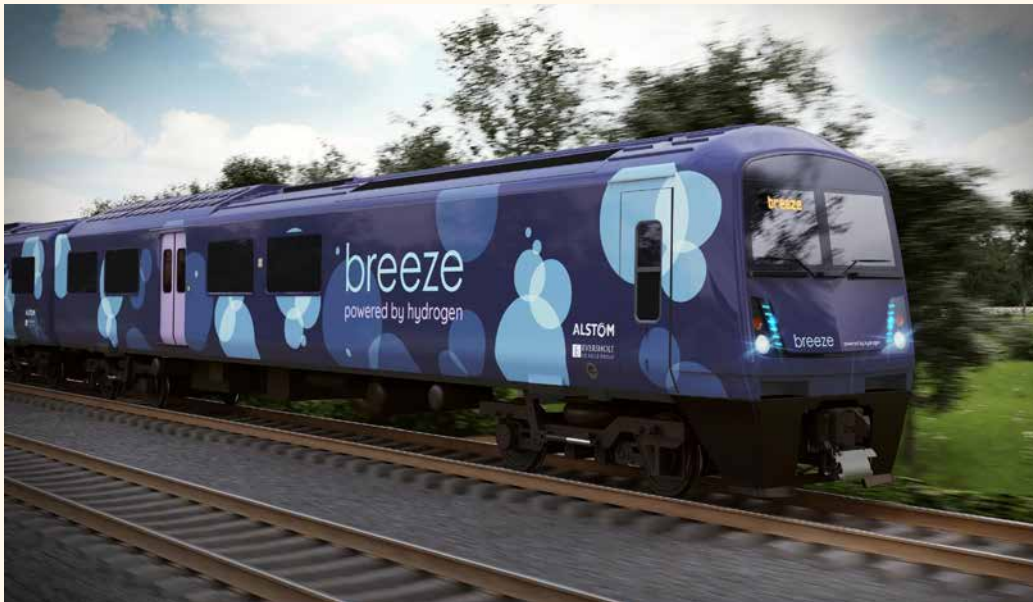
Figure 14 – The hydrogen 'Breeze' train developed by Alstom and Eversholt Rail
