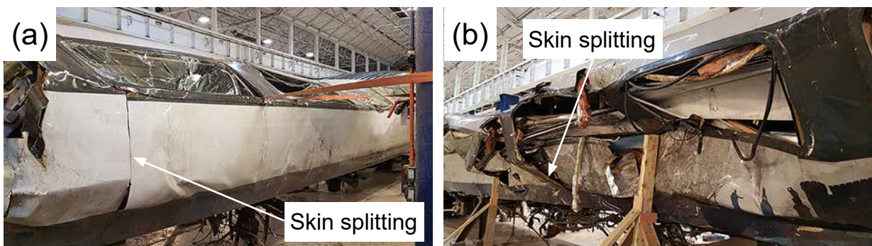
Figure 82: Bodyside skin splitting on coach D, left side (a) and right side (b)
