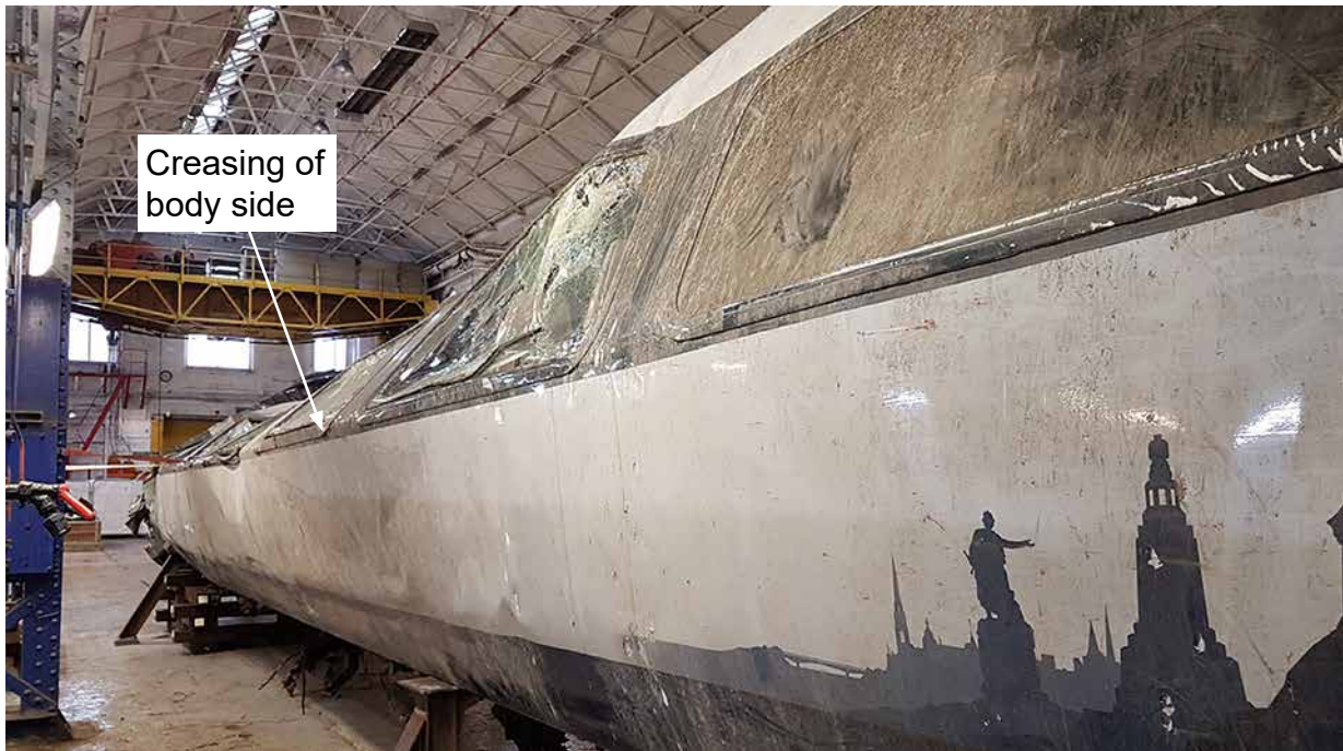
Figure 81: Creasing along left-hand bodyside of coach D
