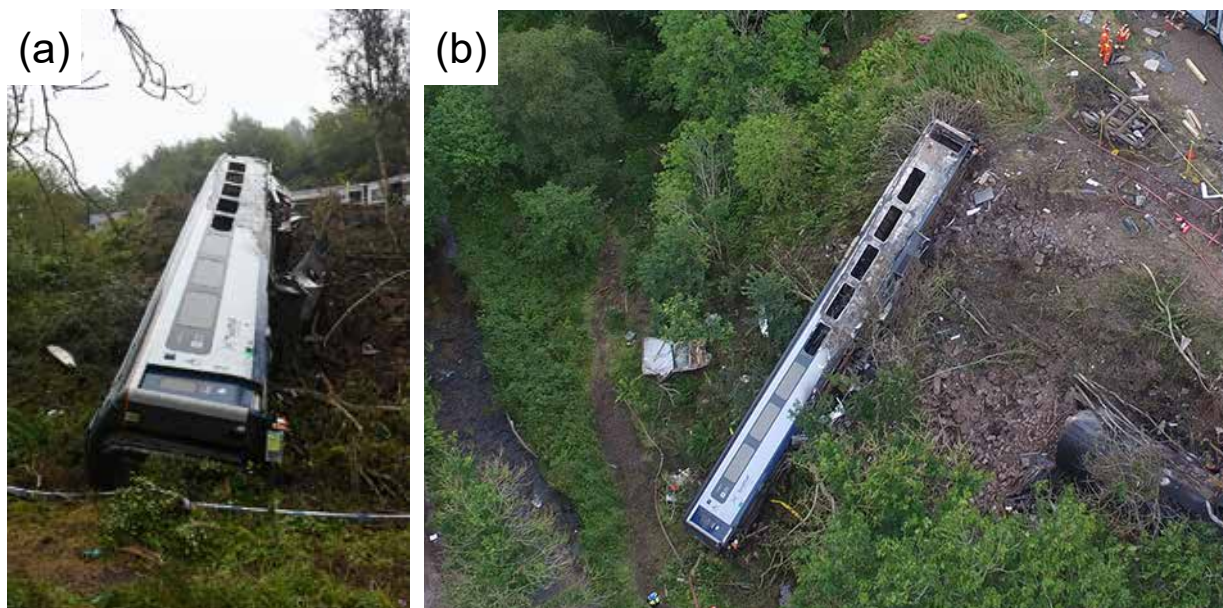
Figure 91: Coach B showing fire damage viewed (a) from bottom of embankment and (b) from overhead
