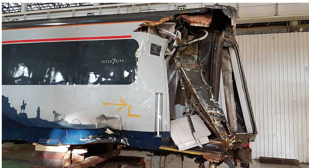
Figure 79: Damage to leading end of coach A
