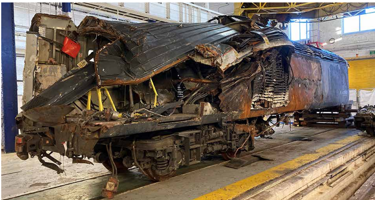
Figure 87: Fire-damaged leading power car
