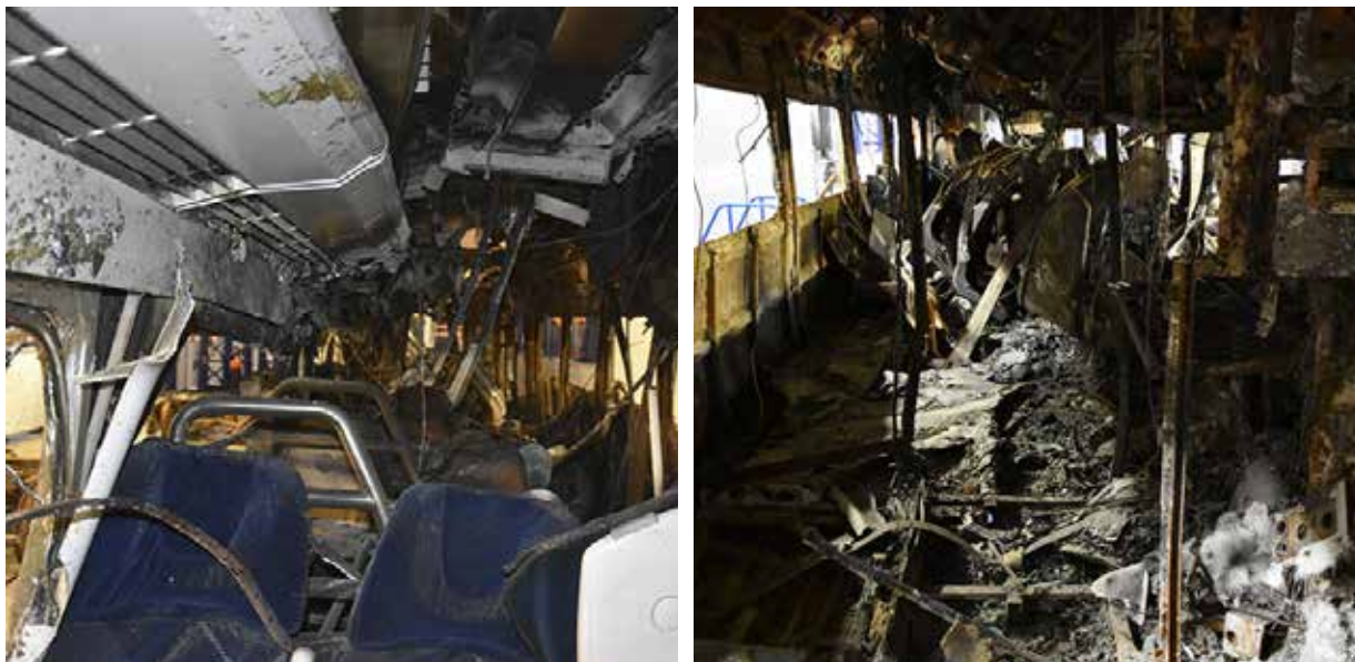
Fire damage in the third coach
