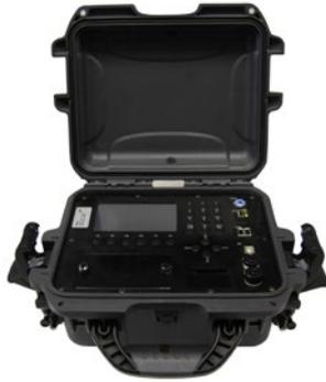
Testing device for track balises. It can test track balises made by any producer worldwide. It offers contactless frequency measuring and storing the information directly to the internal memory of the device. Long-life accumulator battery enables daylong (up to 12 hours) outdoor measuring.
