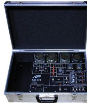
Testing device for central unit of INDUSI I60 (ALTPRO, Siemens, SEL) based ATP system. It can simulate all actual working conditions in order to test them. There is a possibility to test with external or internal (integrated) locomotive balise.
