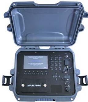
Testing device used for track balise control which is capable of generating short impulse while track balise is active (the rest of time test track balise) or inactive. The width of that impulse is proportional to the travel speed of the train.
