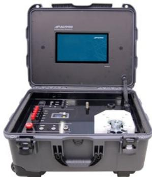
Testing device used for incremental encoder and pick up sensors testing. It is designed to be simple and easy to use for field testing activities.
