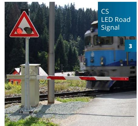
**RLC23 Level Crossing Protection** system is a 2 out of 2 SIL4 certified system. ALTPRO is producing all system components (central device, train detection, barriers and signals) which enables the Customer maximum flexibility. RLC23 is a highly configurable system and can be easily adapted to any requirement set by the Customer.
