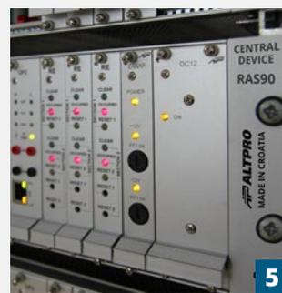
**RAS 90 (PZB90)** system consists of central device **RAS90**, locomotive balise, track balises and signalling and operating elements located in the locomotive cabin. The system offers high level of reliability and safety while maintaining the main idea of ALTPRO INDUSI based ATP systems - simplicity, robustness and longevity.
