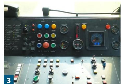
**AUTOSTOP (I60)** system consists of central device **RAS8385**, locomotive balise, track balises and signalling and operating elements located in the locomotive cabin. It is a simple, robust and extremely reliable system. ALTPRO can offer any service/product related to this system from project documentation all the way to system commissioning.
