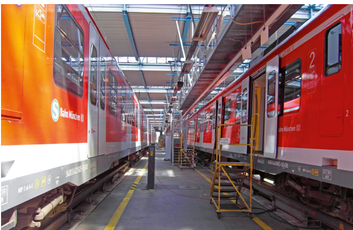
Safely working on the vehicle roof: TracFeed® AEA ensures that the catenary is shutdown and earthed before the work is started
